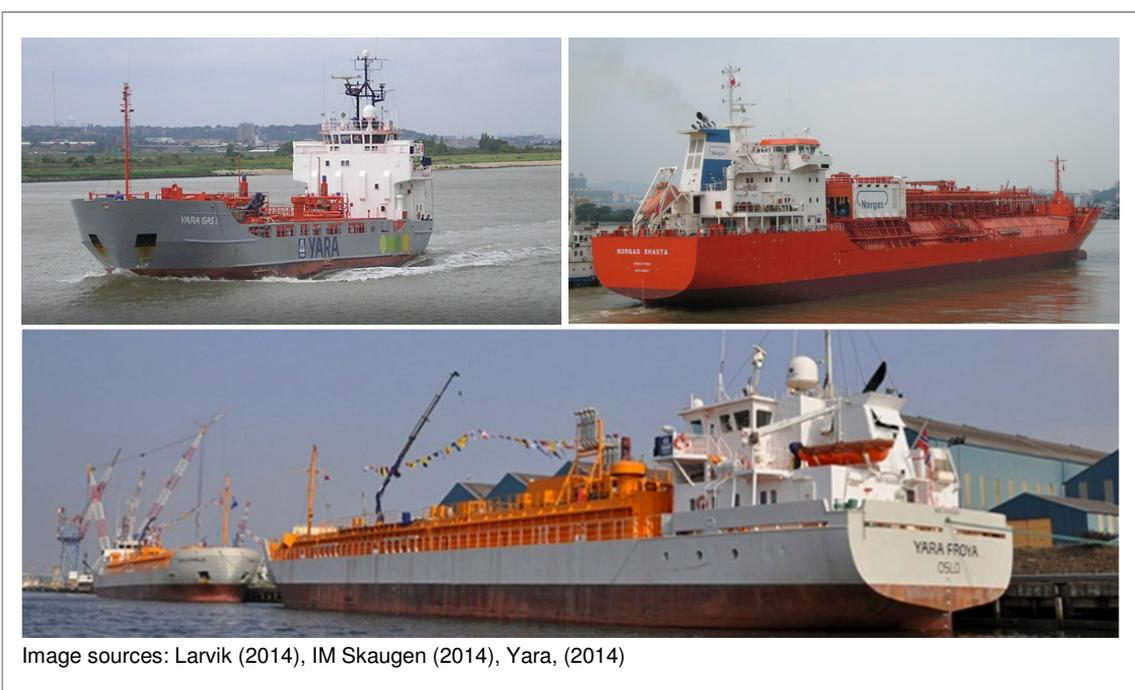
**Figure 4. Examples of existing CO<sub>2</sub> and dual-purpose LNG/CO<sub>2</sub> carriers**
