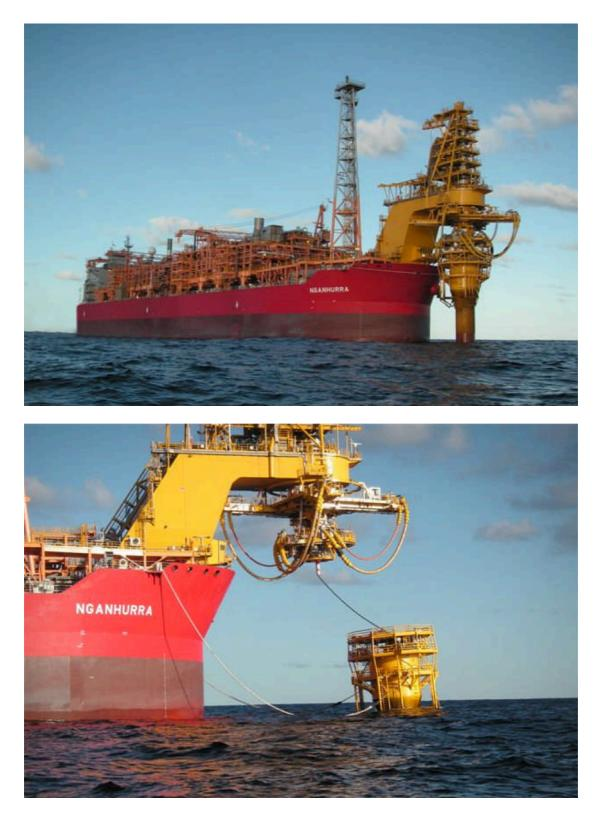
Figure K. Disconnectable external turret mooring. Source: Smith (2009)
