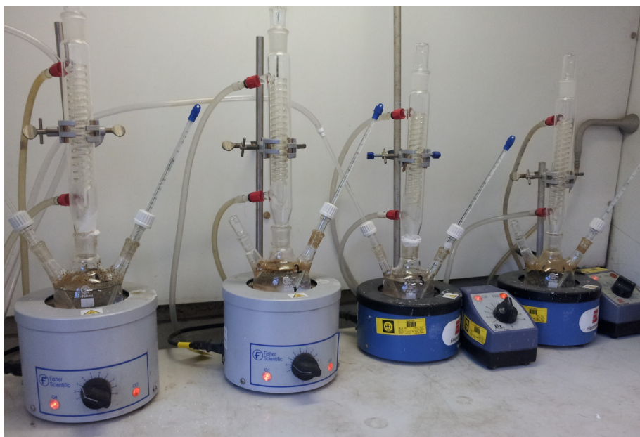
Figure 8. CO 2 batch experimental setup. Flasks are F1-F4, left to right. Flasks F1 & F2 contain sample 8518; flasks F3 & F4 contain sample 8579.
