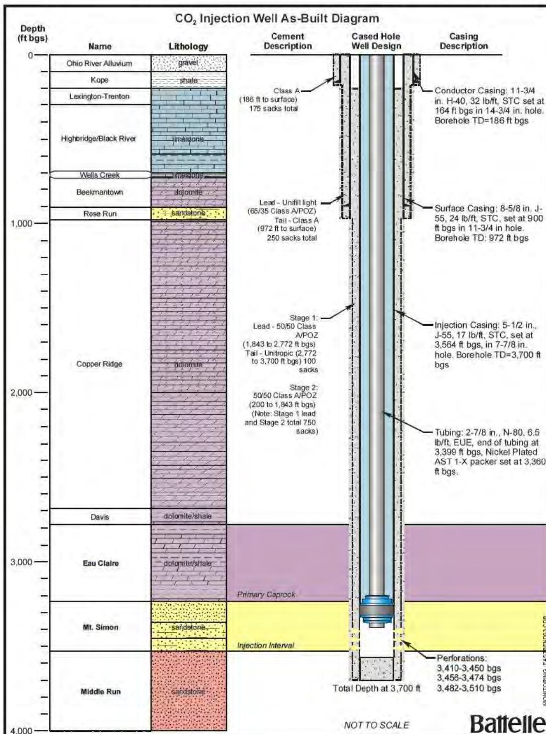
**Figure 14.** Sedimentary column at the MRSP East Bend site of injection (from <http://216.109.210.162/CincinnatiArch.aspx>).
