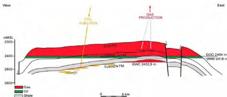
**Figure 47.** Stratigraphy and structure of the Snohvit CO<sub>2</sub> injection site (from Torp). Depth in metres below mean sea level (mMSL). GOC – Gas-Oil Contact. OWC – Oil-Water Contact.
