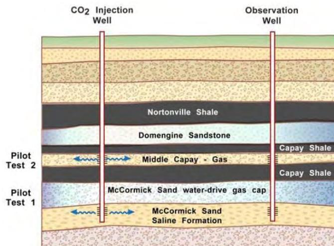
**Figure 21.** Typical geological cross-section showing stacked reservoir and the targeted sedimentary formations: McCormick Sand and Middle Capay Shale, WESTCARB Rosetta injection site (from Trautz et al., 2006).
