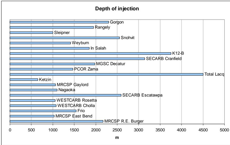
**Figure 2.** Depth of injection, in metres.
