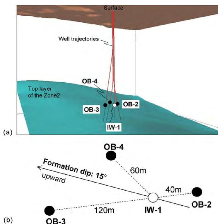
**Figure 25.** (a) Configuration of the injection well (IW-1) and observation wells (OB-2, -3, -4) (b) Plan view of well locations at the top of high porosity injection layer at Nagaoka CO<sub>2</sub> injection site (from Mito et al., 2008).
