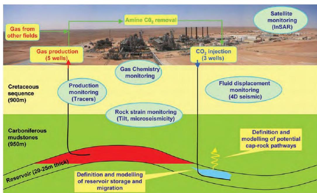
**Figure 42.** Summary of the In Salah CO<sub>2</sub> injection and storage site at Krechba with the main monitoring activities (from Ringrose et al., 2009).
