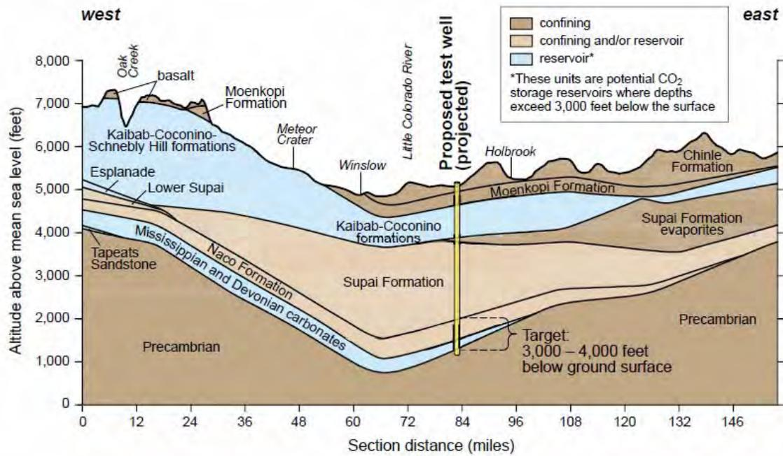
**Figure 18.** East-west regional schematic geologic cross-section of the WESTCARB CO<sub>2</sub> sequestration pilot project (from Shirley et al., 2009).
