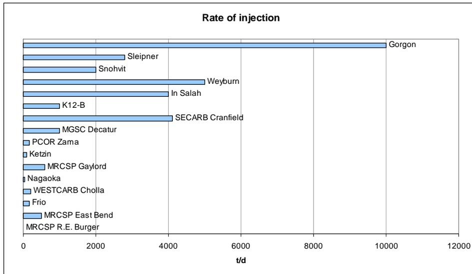
**Figure 8.** Daily rate of injection, tonnes CO<sub>2</sub> per day.
