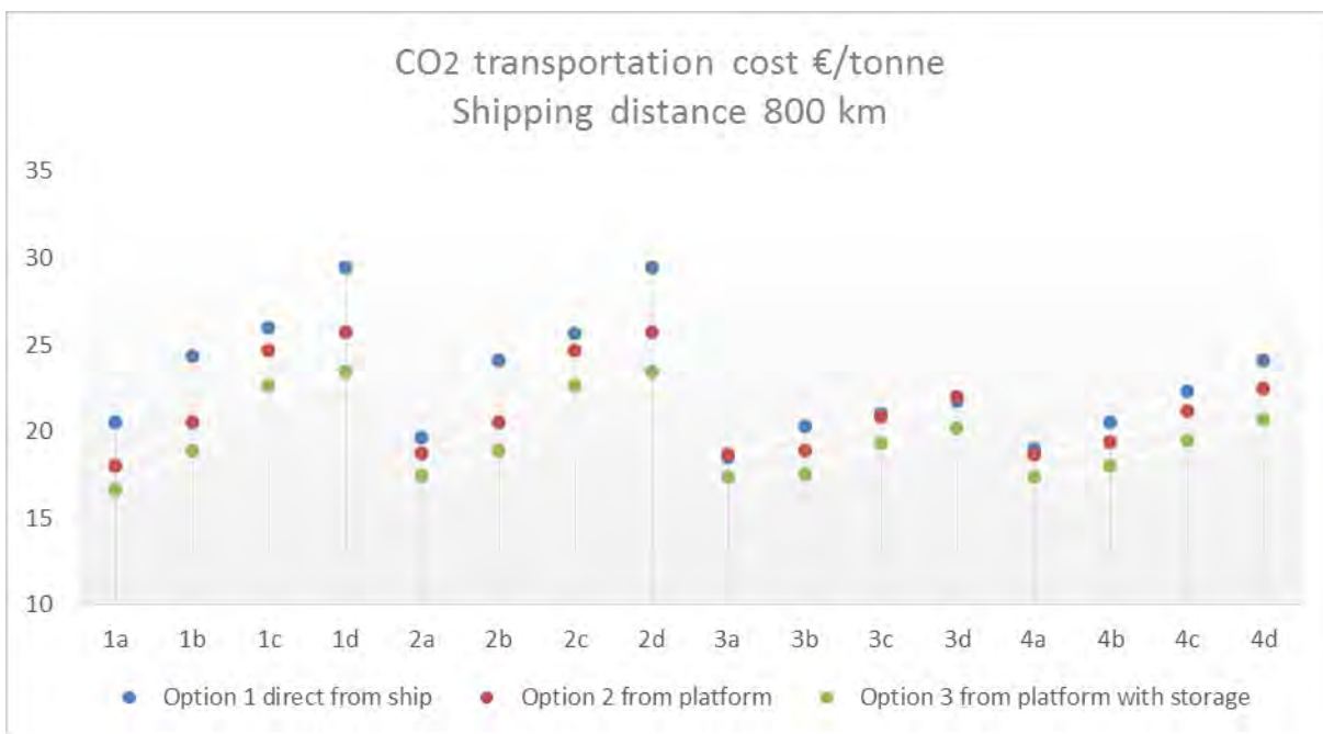
Figure 6-3: CO 2 transportation cost for the different reservoir cases at a shipping distance of 800 km
