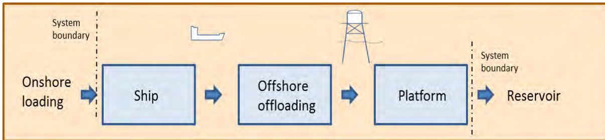
Figure 3-3: Second design option: CO 2 shipping to an offshore offloading point close to the injection site and injection from the platform. No intermediate offshore storage. CO 2 processing both on the ship and platform.
