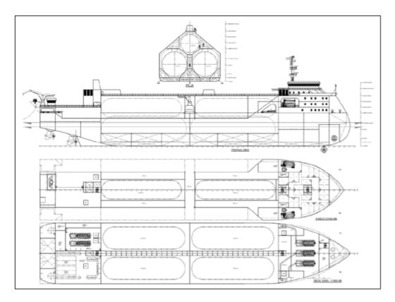
Figure 6. General arrangement of proposed X-Bow design 30,000m<sup>3</sup> CO<sub>2</sub> carrier (Vermeulen, 2011)
