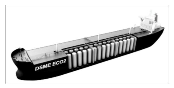
Figure 7. Conceptual drawing of 100,000m³ very large CO<sub>2</sub> carrier (Yoo et al, 2013)
