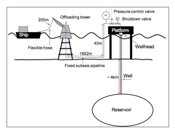
Figure 11. Fixed tower single point mooring offloading to platform (Vermeulen, 2011)
