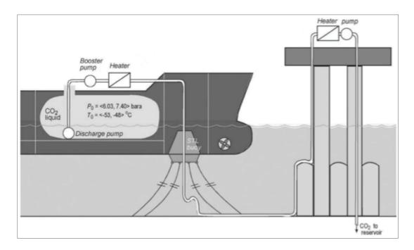
Figure 10. Sketch of submerged turret loading system (Aspelund, Mølnvik and de Koeijer, 2006)
