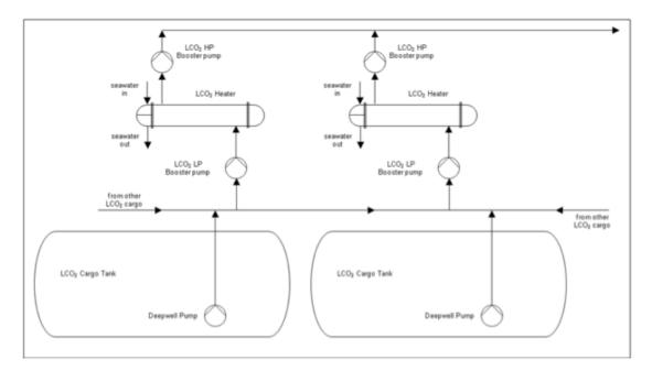
Figure 8. Proposed discharge equipment on ship (Vermeulen, 2011)
