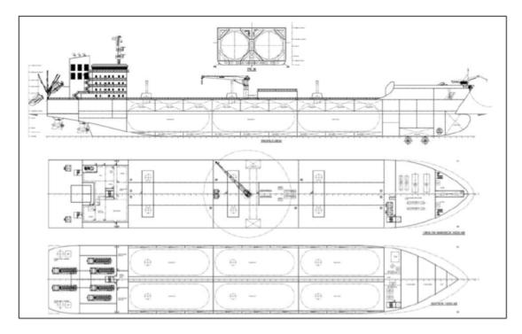
Figure 5. General arrangement for proposed 30,000m<sup>3</sup> CO<sub>2</sub> carrier, conventional design (Vermeulen, 2011)
