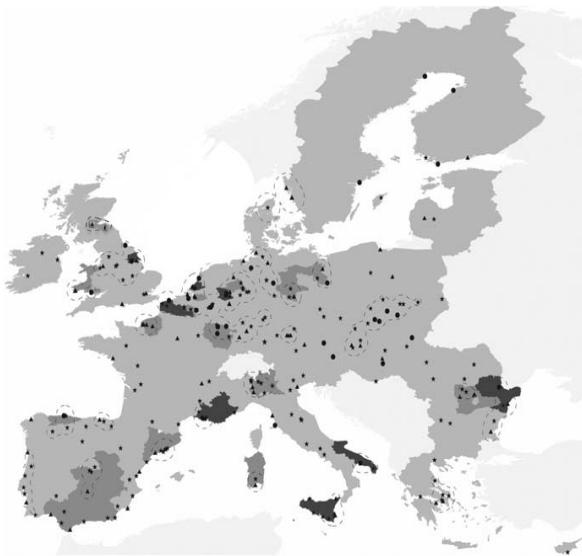
Key: ▲ refineries, ● integrated steel plants, ★ cement plant Mid grey: regions with large industry sources totalling >5 Mt/yr, Dark grey: regions totalling >10 Mt/yr, Pecked lines: potential capture clusters. Adapted from: Rootzén, et al, Management of Environmental Quality, 22, (1), 2011
