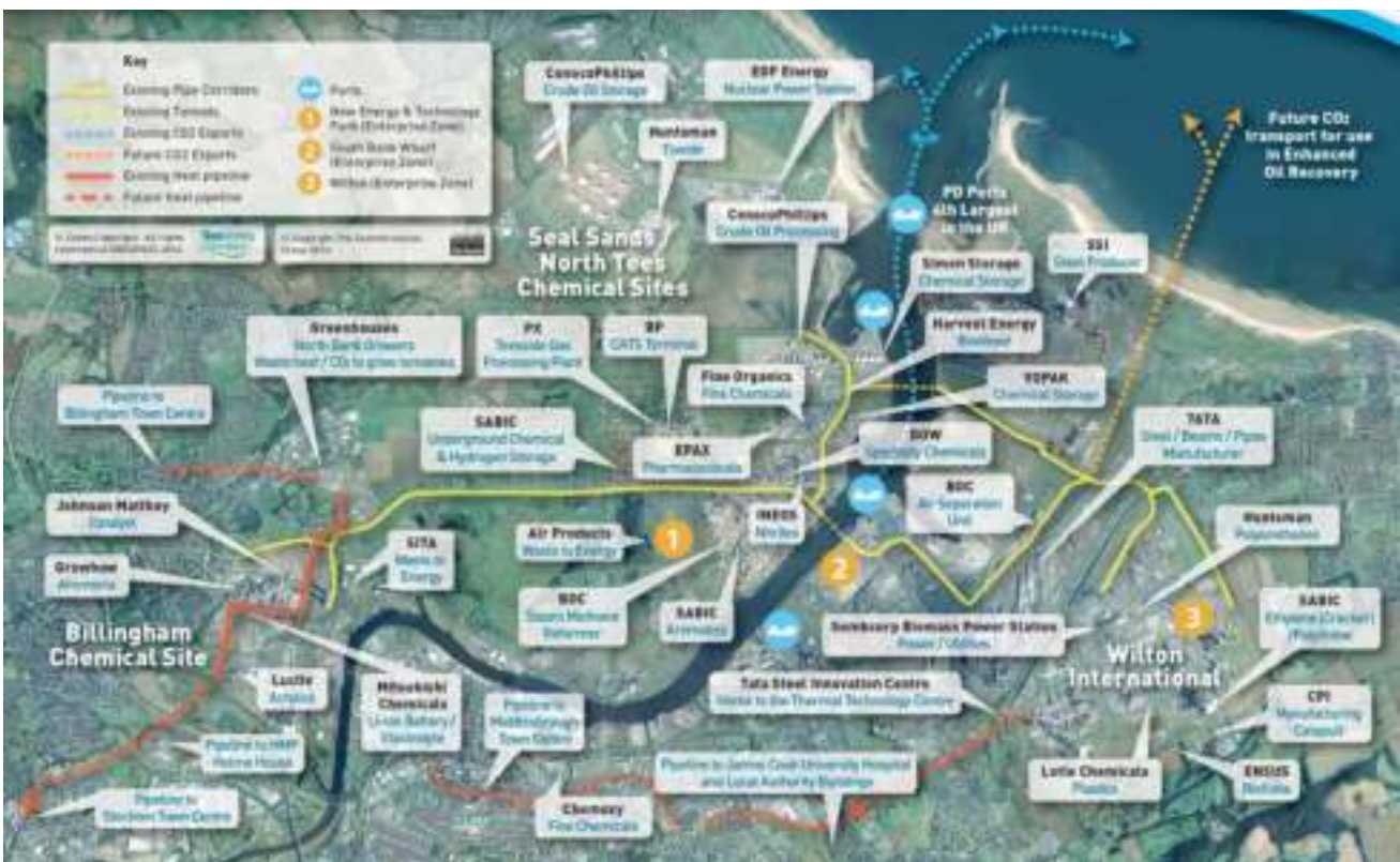
Figure 6: The proposals for Tees Valley consider several CO 2 capture points, including SSI's steel blast furnace (3–5 Mt per year) and Growhow's fertiliser plant (0.6 Mt per year). Source: Tees Valley Unlimited
