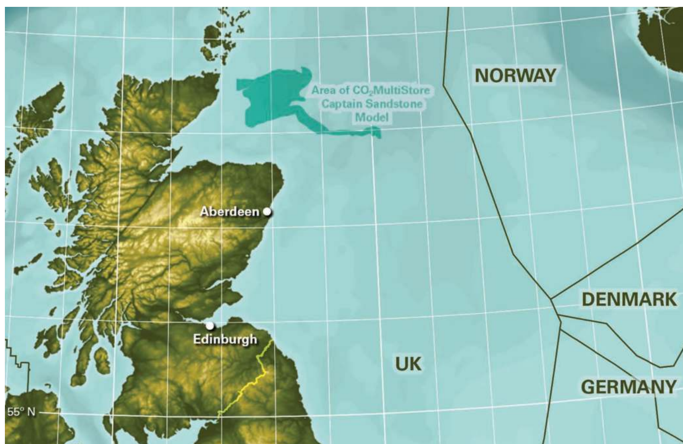
Figure 2: Potential CO 2 storage sites beneath the North Sea include the Captain Sandstone, which is one of the best understood offshore sites due to decades of oil and gas sector operations. Source: British Geological Survey
