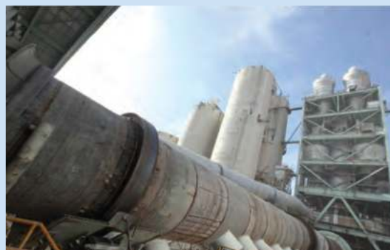
One third of CO 2 emissions from a cement plant derive from fuel combustion and two thirds from the calcination process itself. Photo: LafargeHolcim 2015
